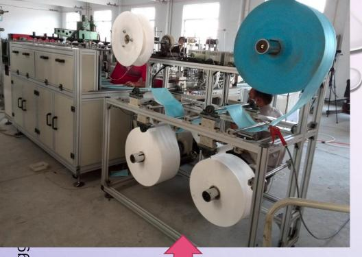
Mask making line with ear-loop welding on-line
