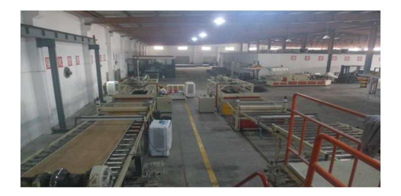
The production process is simplified as the extrusion Plus Calendaring of PVC+CaCO3 with additives, makes the base upon which decorative PVC film and wear layers [ 200 to 500 Micron thick] are hot-laminated on-line, then UV Coated and then slit in to needed sizes and then Milled for the edges to make them coupled in to each other while lying on {A sort of Male-female coupling}
