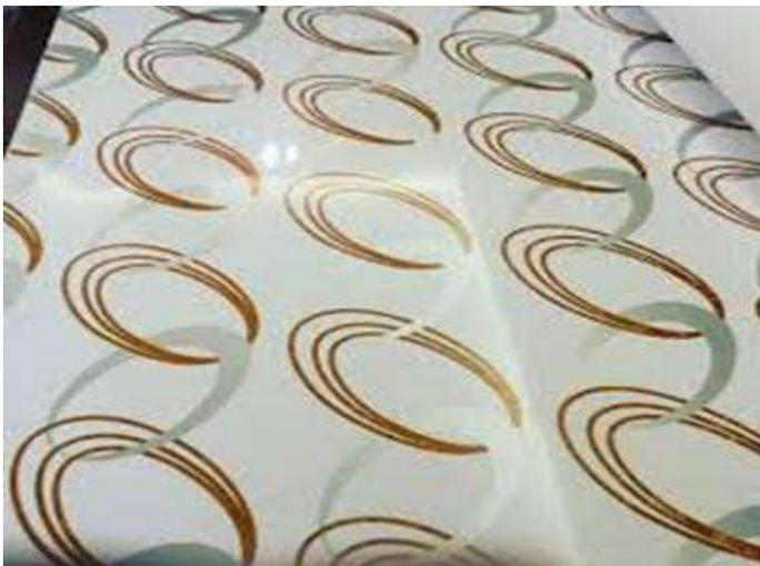
This is made from PVC + CaCO<sub>3</sub> and additives and can be made unbreakable upon bending many times. This product proves much cheaper to be used as core adding higher amount of CaCO<sub>3</sub> (this is breakable) This avoids use of formaldehyde and paper and is pollution free.
