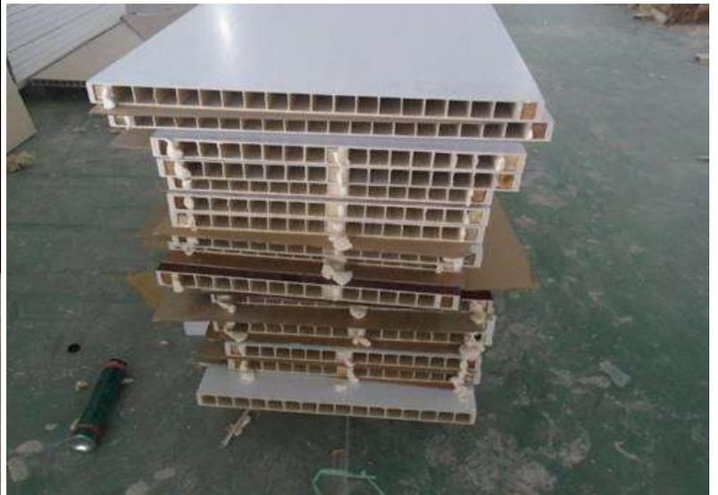
Made from Wood plus PVC and additives, this product is again termite-proof and water-proof needing almost nil maintenance, not much of wood working, can be made available ready-made without the need of any sort of carpentry on it, no color and no varnish. Still if the need be, can be colored. This product can save much of wood.
